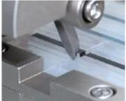
It is designed to notch specimens for Charpy & Izod impact tests. 20 specimens may be clamped at one time and at least 100 specimens may be notched in 10 minutes. It allows a perfect reproducibility of the notches, increases working efficiency and reduces the labor intensity.
