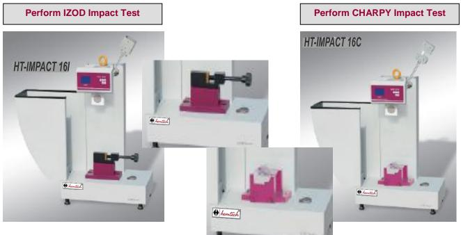
Models available with combined Testing as well. Combined Model can perform Testing for IZOD & CHARPY both using the same Instruments. It comes with Vice & Hammers for Izod and Charpy.
