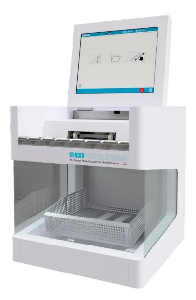
The operation of the system is easy enough that any operator can do it. The Filmtest helps to reduce the work in the laboratory. For example, in addition to the thickness measurement, the unit weight of the sample is also calculated eliminating the manual step of weighing the film.
