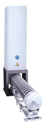
The RCP tester conveniently and accurately determines the critical pressure and critical temperature for rapid crack propagation in PE pressure pipes.
